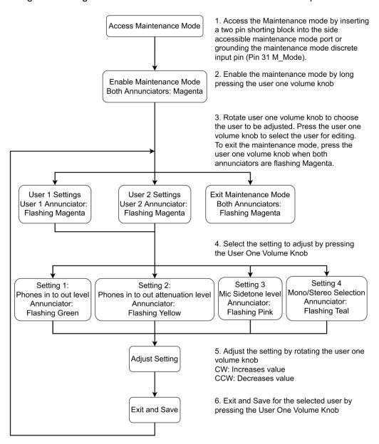
Figure 13: Field Adjustable Maintenance Mode Flowchart
