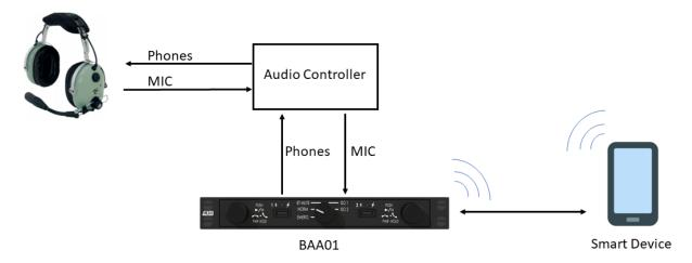
Figure 3: BAA01 in a Transceiver Position
