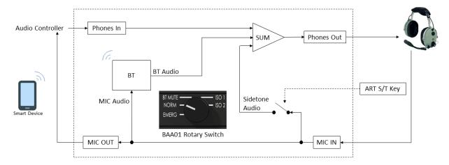
Figure 7: Normal Audio Routing
