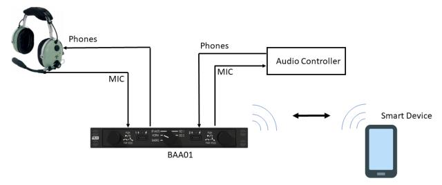
Figure 2: BAA01 In-Line between the Headset and Audio Controller
