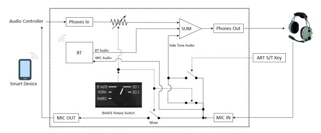
Figure 9: Isolate Audio Routing
