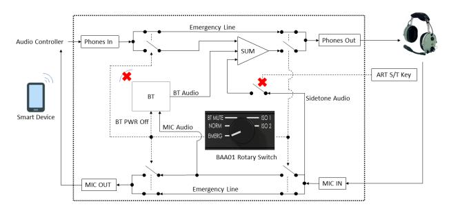
Figure 6: Emergency Audio Routing
