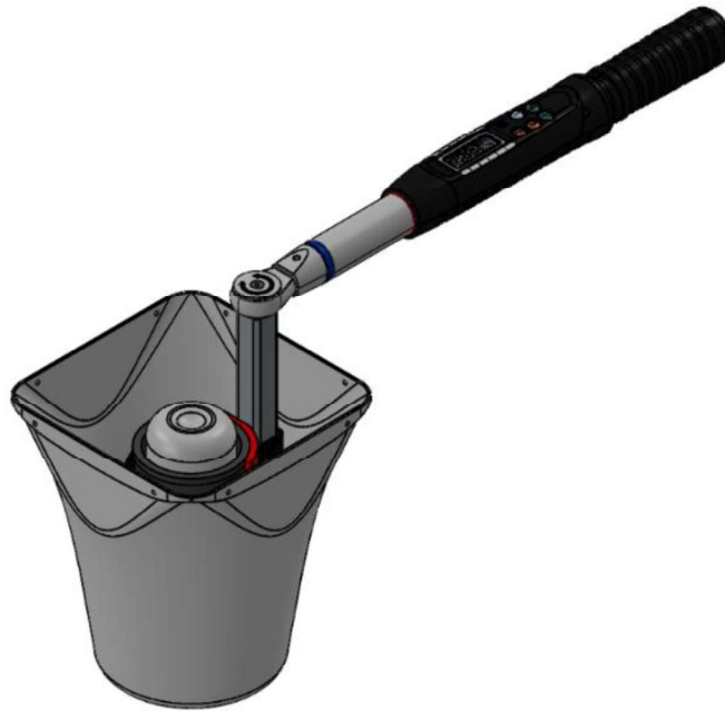
Figure 12 – Re-Entrant Tip Inspection with Torque Wrench Assembly
