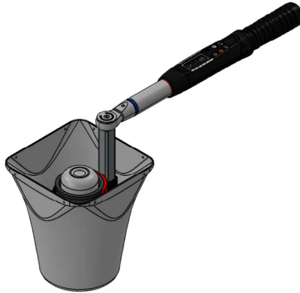
Figure 3 – Re-Entrant Tip Removal with Torque Wrench
