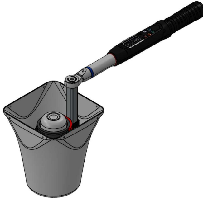
Figure 9 – Re-Entrant Tip Reassembly with Torque Wrench
