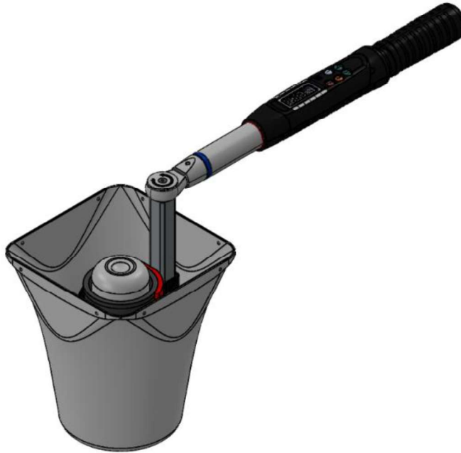
Figure 12 – Re-Entrant Tip Inspection with Torque Wrench Assembly
