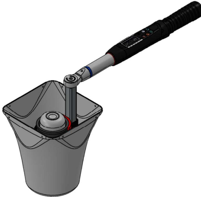
Figure 9 – Re-Entrant Tip Reassembly with Torque Wrench
