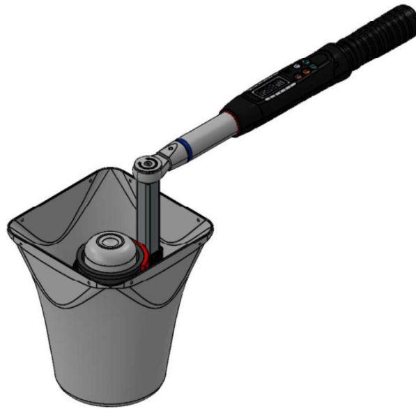
Figure 3 – Re-entrant Tip Removal with Torque Wrench
